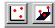
Figure 2.3. Graphic speed buttons for the EIGEN module. The first button calls MXPLOT to produce a 2D plot of the eigenvectors and the second calls MOD3D for a 3D plot.
